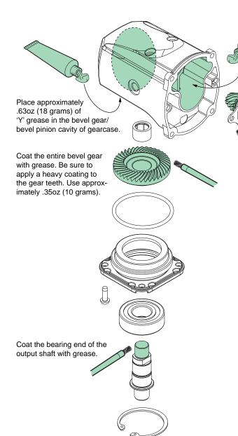
Place approximately .70oz (20 grams) of 'Y' grease in the gearcase cavity for the armature pinion and intermediate gear assembly.
