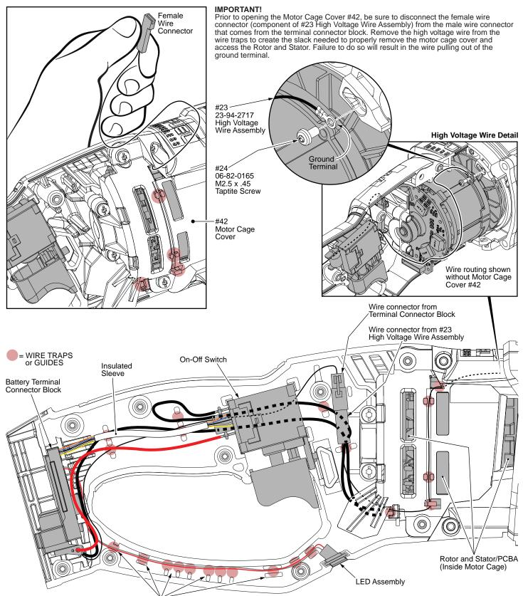
16 Wire Ribblon Cable from Terminal Connector Block to the PCBA is not shown for clarity. Ribbon Cable is routed over the LED Assembly wires using the same traps.
